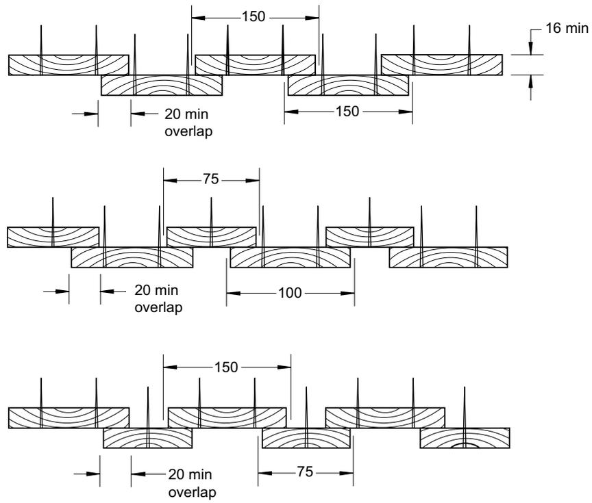
Figure 5.18 Profiles suitable for vertical boarding
