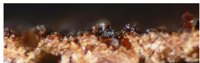
Figure 7 Transverse section taken from surface of western red cedar cladding with severe extractive staining, showing dark-coloured extractives confined to the surface zone
